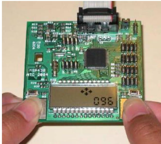
Figure 3. ECG monitor based on MSP430FG439 microcontroller.
